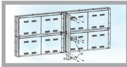
2. Assemble cabinets to steel frame
